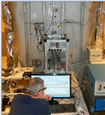
Henrik Svensmark uses the gamma-ray irradiated chamber in the background to pinpoint the mechanism linking atmospheric ions and cloud condensation nuclei.
