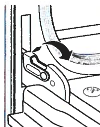
Pull hinge: locks up to unlock
