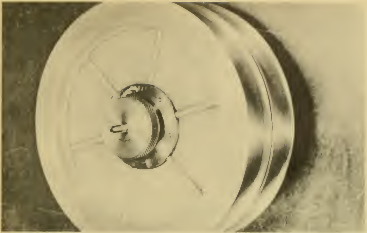
Photograph 3a. High speed wire drive No. 3; wire reels in place.
