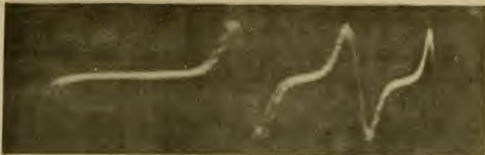
Output voltage direct from reading head. Three similar pulses spaced 141 to the inch. Recording pulse duration 8 microseconds, peak recording current 6.3 milliamperes.
