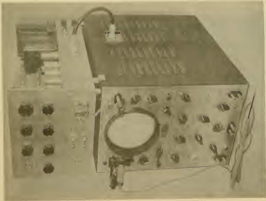
Figure 26 Fast Sweep, Marker, and Delayed Trigger Generator (shown in place on oscilloscope)
