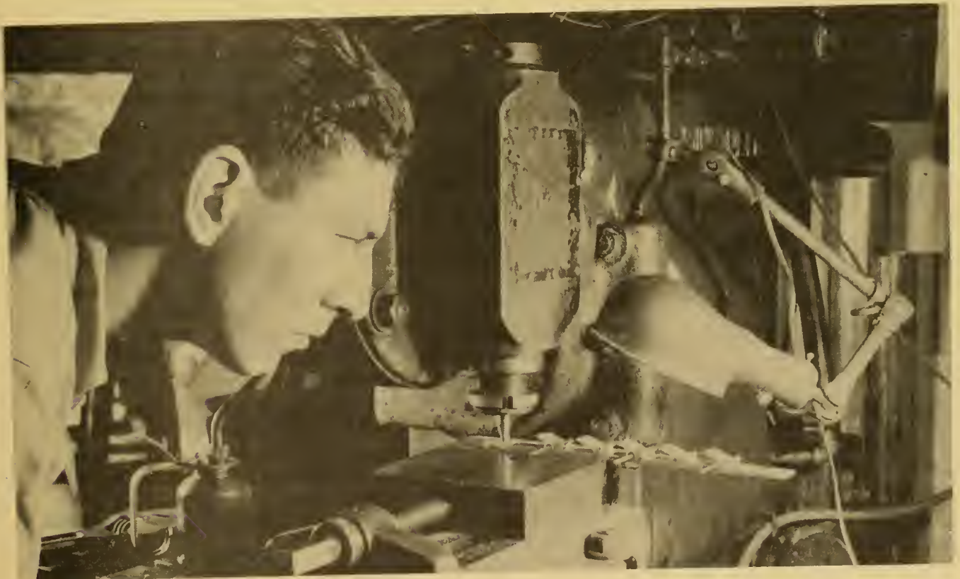
Photograph 7-b Fabrication of Copper Strips for Sandwich
