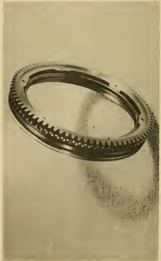
Photograph 14-c Worm Gear, Steel Track, and Slip Rings of Slow Drive
